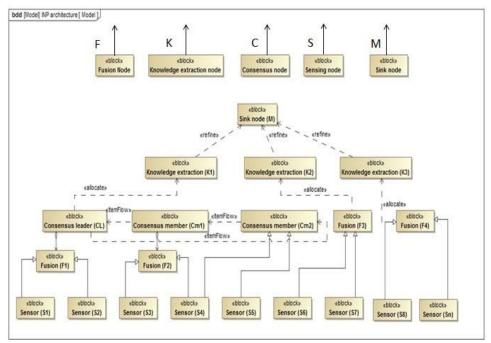
ity of smoke and fire detection. One of the most obvious examples is receiving the input of a number of 'S' nodes and fusing them using some unsupervised learning method, e.g. PCA, k-means, etc., for dimensionality reduction.
